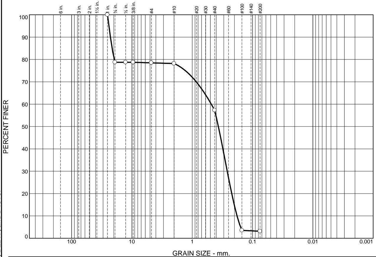
ASTM Specifications performed my include: D421, D422, D2216, D2217, and D4318.
